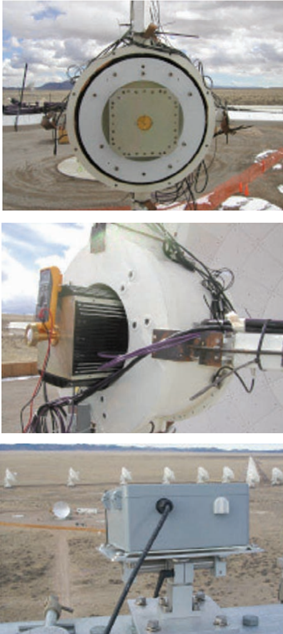
Fig. 6.7. The hardware configuration: signal feed side of the receiver (top), reference feed side of the receiver (middle) and transmitter on top of tower aiming at the antenna in foreground. The other antennas are part of the NRAO Very Large Array in New Mexico.
