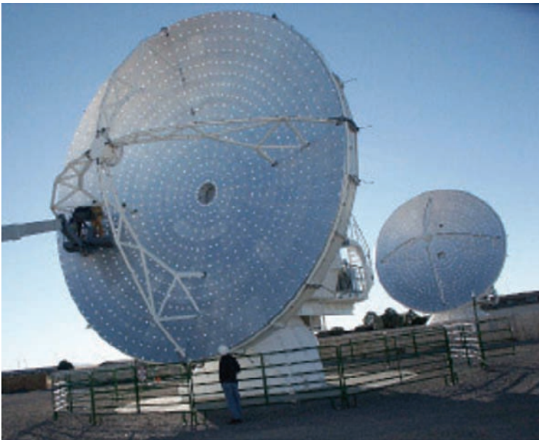
Fig. 6.11. The ALMA prototype antennas are covered with 1080 photogrammetry targets, placed in 17 rings of 24 - 96 targets (white dots).
