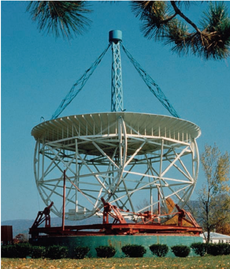
Fig. 1.1. Reber's 10 m antenna, reconstructed at the National Radio Astronomy Observatory, Green Bank, WV, USA. The original dish did not have the azimuth movement; it was a transit instrument. (NRAO/AUI/NSF)
