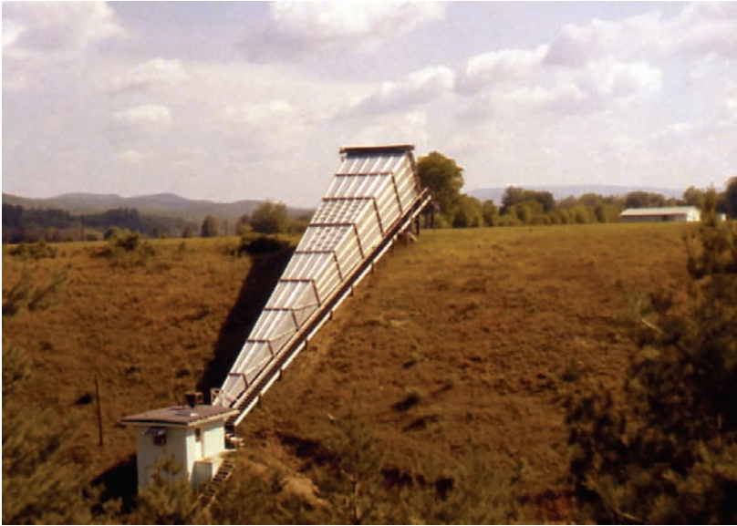
Fig.1.10. The 25 m long "Little Big Horn" at NRAO, Green Bank, used for absolute flux density measurements of Cas A at 1400 MHz over many years. The rotation of the earth carried the source through the beam once a day. (NRAO/AUI/NSF)
