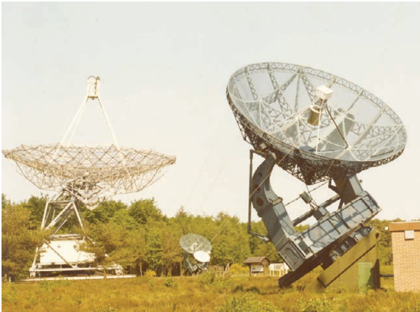
Fig.1.2. A 7.5 m diameter "Würzburg" antenna, mounted equatorially (foreground) at the Dwingeloo Radio Observatory, Netherlands. The 25 m telescope is in the background. Both antennas were used as an interferometer in an experiment described in Ch.6.2. (Henk Snijder, ASTRON)
