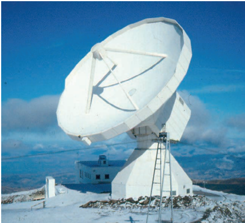
Fig. 7.11. The IRAM 30-m Millimeter Radio Telescope (MRT) at 2850 m on Pico Veleta, Spain. The collar on top is to avoid ice falling from the rim onto the reflector. The reflector itself can be heated from the back to avoid ice deposit during icing storms. (Photo by the author, IRAM)
