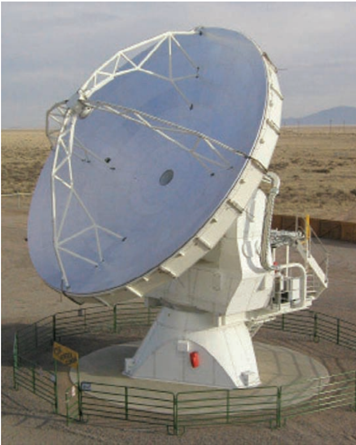
Fig. 7.21. Prototype 12 m diameter antenna for ALMA, designed and built by VertexRSI. Note the curved quadripod to minimise the spherical wave aperture blocking. (N.Emerson, NRAO/AUI)
