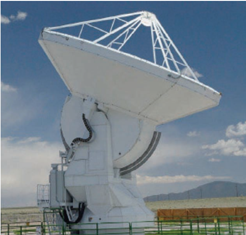
Fig. 7.22. Prototype 12 m antenna for ALMA designed and built by Actatel - European Industrial Engineering Consortium. This antenna employs direct drives with linear motors. The magnet arc of the elevation drive is well visible. (N. Emerson, NRAO/AUI)
